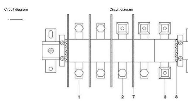
1 = high current connector, AS screw set on both sides
