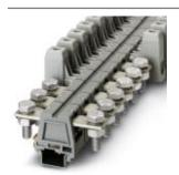
Universal terminal block with bolt connection, cross section: 25 - 50 mm², AWG: 6 - 1/0, width: 32 mm, color: gray
