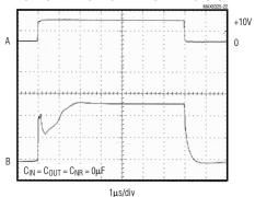
A: V<sub>IN</sub>, 10V/div B: V<sub>OUT</sub>, 1V/div
