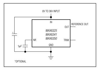
Figure 2. Noise-Reduction Capacitor
