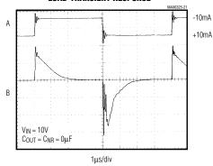
A:  $I_{OUT}$  ( $\pm 10$ mA SOURCE AND SINK), 20mA/div, AC COUPLED B:  $V_{OUT}$ , 20mV/div, AC COUPLED
