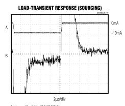
A:  $I_{OUT}$ , 10mA/div (SOURCING) B:  $V_{OUT}$ , 500 $\mu$ V/div
