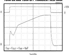
A: V<sub>IN</sub>, 10V/div B: V<sub>OUT</sub>, 1V/div
