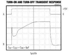
A: V<sub>IN</sub>, 10V/div B: V<sub>OUT</sub>, 1V/div
